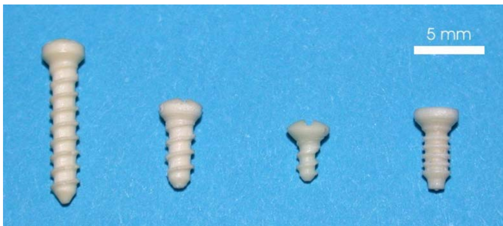
Fig. 1 Examples of developed and studied multifunctional bioabsorbable drug-releasing hard tissue fixation devices including from left to right screws, miniscrew and tack
